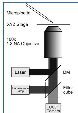
Fig. 3 The experimental setup. The femtosecond laser pulses are introduced in the optical axis of our inverted microscope with a dichroic mirror (DM) and then focused on the sample with a 100x high NA objective. The same objective is used to image the specimen in bright field or epifluorescence microscopy onto a CCD camera.
