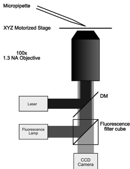
Figure 3. The experimental setup. The femtosecond laser pulses are introduced in the optical axis of our inverted microscope with a dichroic mirror (DM), and then focused on the sample with a 100x high NA objective. The same objective is used to image the specimen in bright field or epifluorescence microscopy onto a CCD camera.
